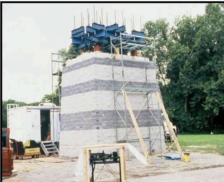
FHWA-TFHRC GRS BRIDGE PIER LOADED TO 10 TSF M. Adams
